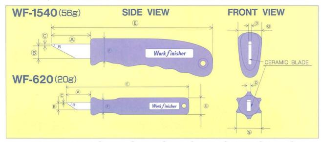
DIMENSIONS: WF-1540 R:30° @:40mm @:14mm @:1mm @:1.5mm @:175mm @:14mm WF-620 R:30° A:25mm B:5mm D:1.5mm E:133mm F:10mm D:14mm
